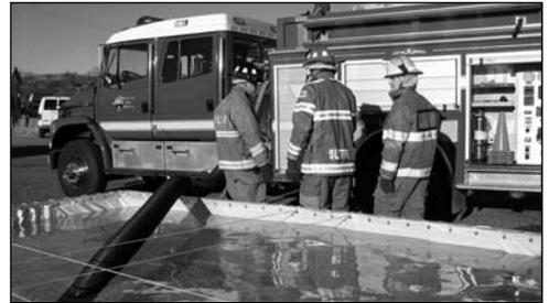
*An engine drafts water from a 3000-gallon portable tank during a drill.*
